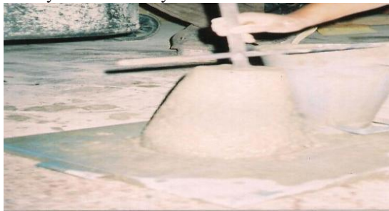
Fig. 2 Slump of concrete
