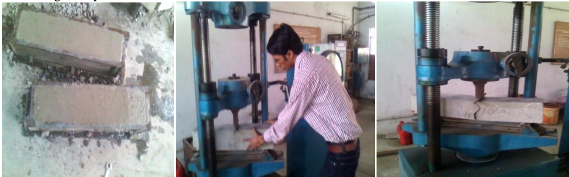
Fig. 5 Testing of concrete beam
