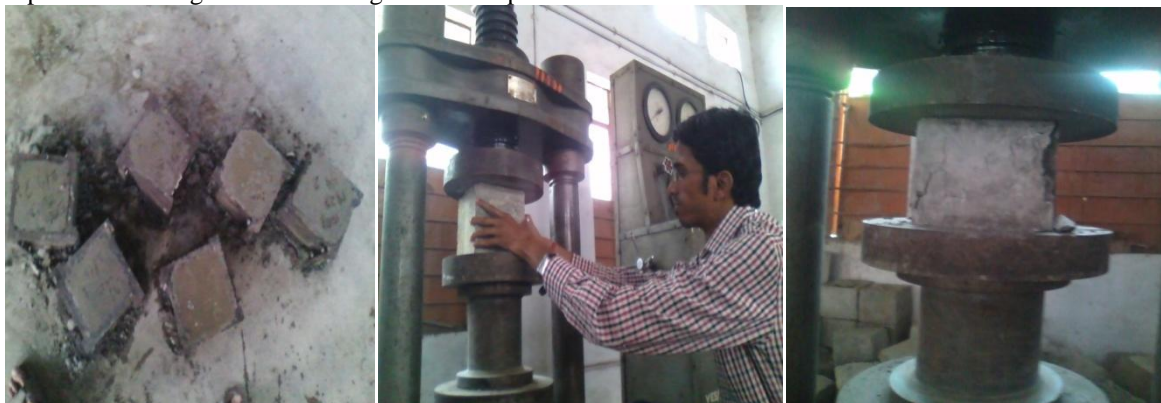
Fig. 3 Testing of concrete cubes
